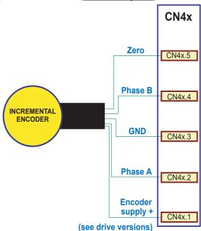
Maximum supply current 20 mA for each encoder (24V version). Maximum supply current 100 mA for each encoder (5V version).
